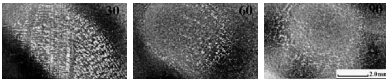
Fig. 15 Wear scars of Stellite X40 under 500 mg/L solids slurry erosion changing angle of impingement
