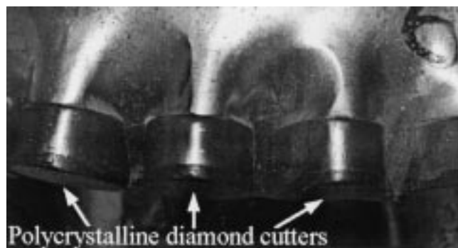
Fig. 1 Severe degradation of the material behind the diamond cutters
